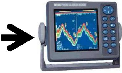
Hydroacoustic survey is just a sophisticated depth sounder that allows fine tuning and logs all the data for further processing. We get a rapid snapshot of summer distribution of the alewife (when people are fishing).
